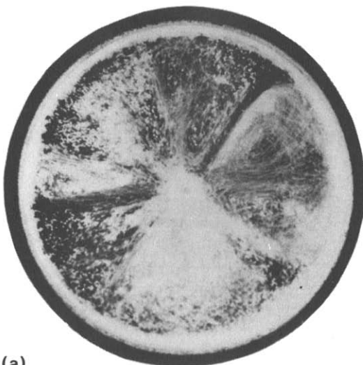
FIG. 1. (a) Streak photograph of electroconvective leaf pattern ( \lambda = 20, v = 30 kV negative). (b) Distribution of radial velocity u , at R_1 < r < R_2 .
